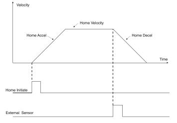
Figure 35: Home to Sensor Profile (Calculated Offset)
